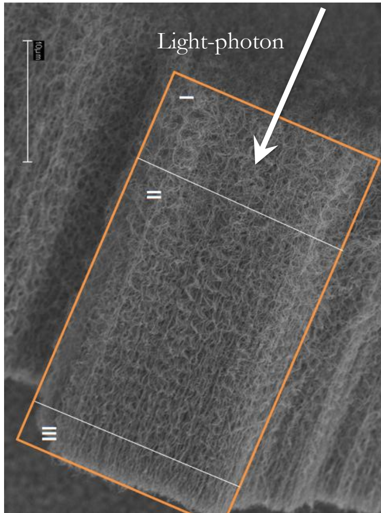
Figure 4.2. SEM image of CNTs with a height of \sim 35 \mu\text{m} . Region I is the surface of the aligned nanotubes which exhibit bridge-like interconnections. Region II shows highly aligned nanotubes with helical growth and Region III is the base where growth begins.
