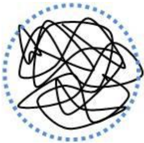
Figure A.6. MWNT bundle with rotational symmetry occupying spherical space.
