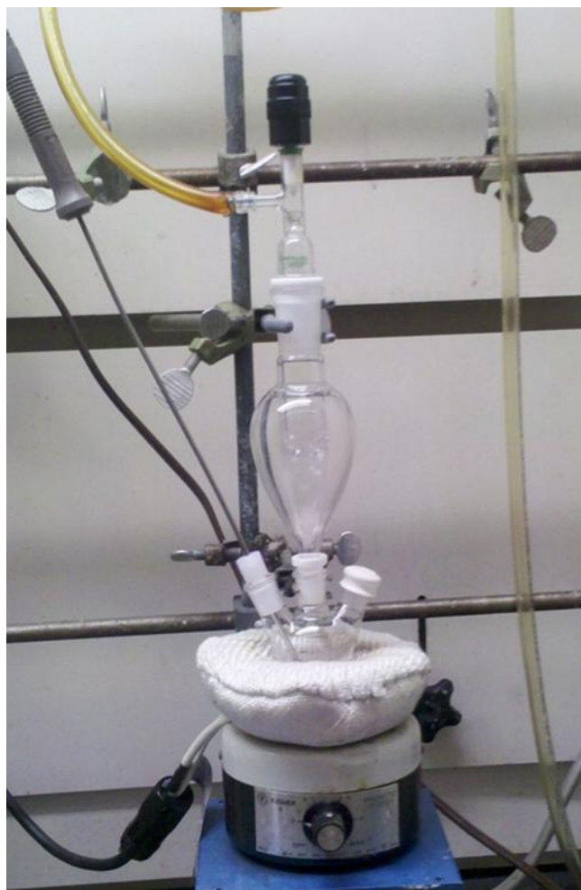
Figure 2.1 Image of nanocrystal synthesis setup. The 3-neck flask was seated atop a stir plate inside a heating mantle, heated to the appropriate reaction temperature. Reaction temperatures are varied by using a digital temperature controller, which is connected to the heating mantle, to set the desired temperature. A thermocouple is also attached to the temperature controller and inserted into the reaction flask to monitor the temperature of the solution. A stir bar was placed inside the flask and stirred rapidly to help maintain a uniform temperature throughout the solution, as well as uniform concentration of reactants. A rotary evaporator, bump trap is inserted into the center neck of the reaction flask and is attached to an argon bubbler to allow the nanocrystal synthesis to occur in an environment free of water and oxygen. The remaining neck is fitted with a rubber septum to close off the reaction to the external environment and maintain synthesis conditions. This neck is also utilizing during anionic precursor injections via syringe.
