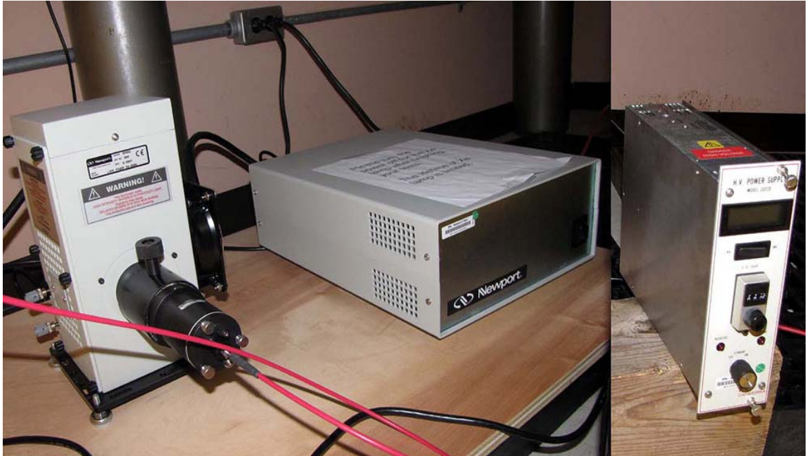
Figure B4. Pockels effect setup. The light source and associated power, as well as the high voltage power supply are seen.
