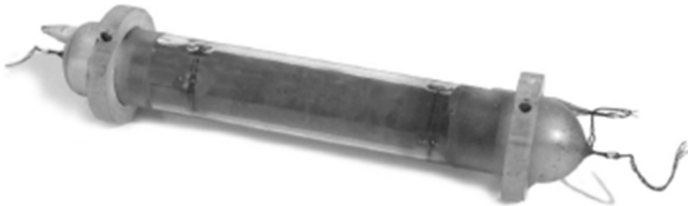
Figure 1.3: Hand-built GM tube with glass wall (1940's). A cylindrical copper tube serves as cathode. The ends of the tube are coated with wax to reduce leakage currents [2].
